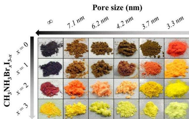
**Figure 1.** Photographs of the mesoporous silica powders after impregnation and crystallization.
